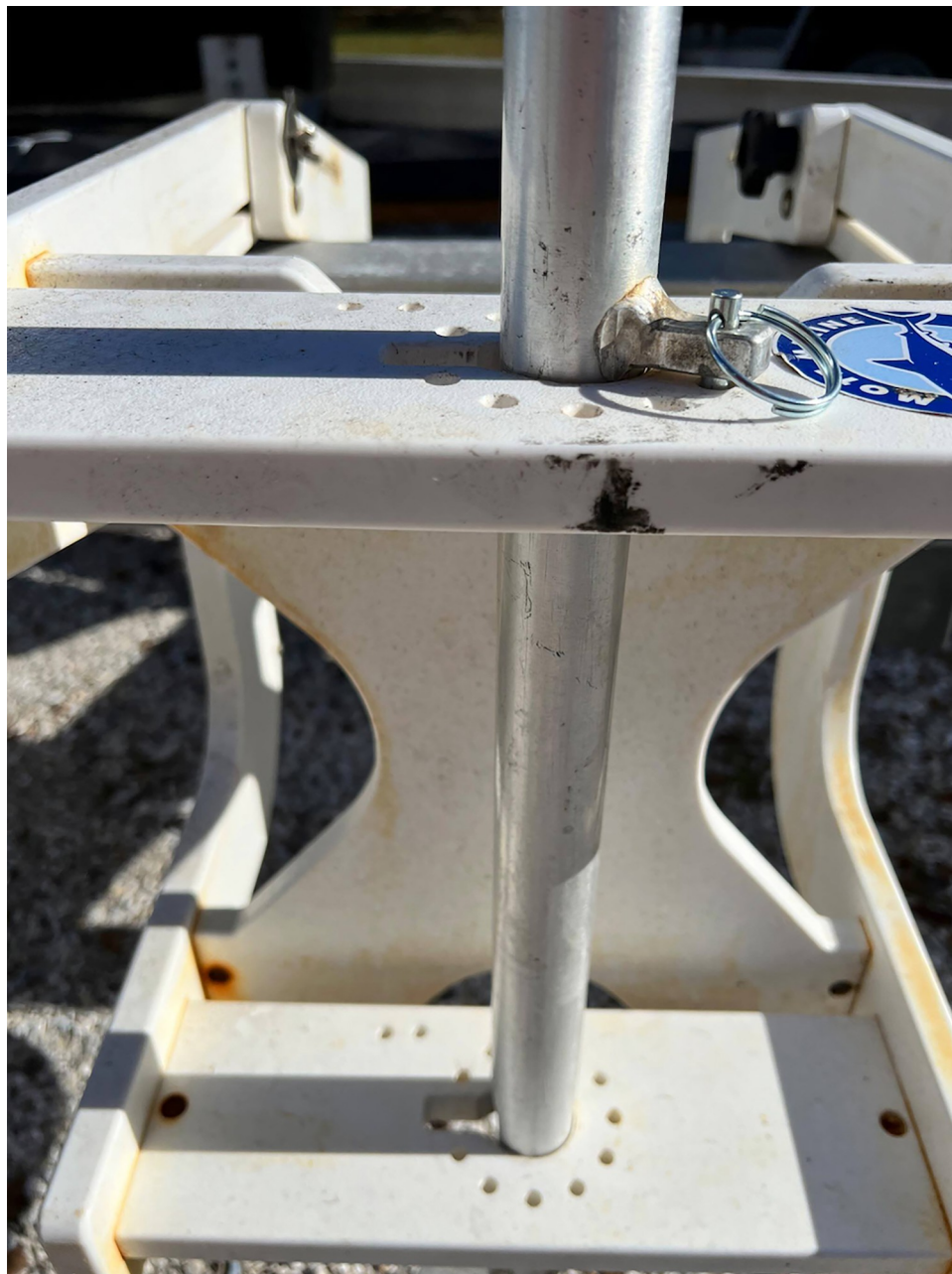
Fig 3. Underwater camera deployment pole positioned through the mount device and secured at a selected depth with a looped stainless steel cotter pin.
