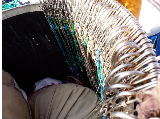
[Fig.13] Fishing gear: 1 drum with approximately 100 hooks on wire trace.
