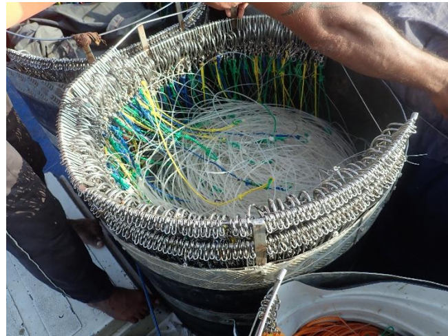
[Fig. 39] Fishing gear, one of three drums with hooks on wire trace.
