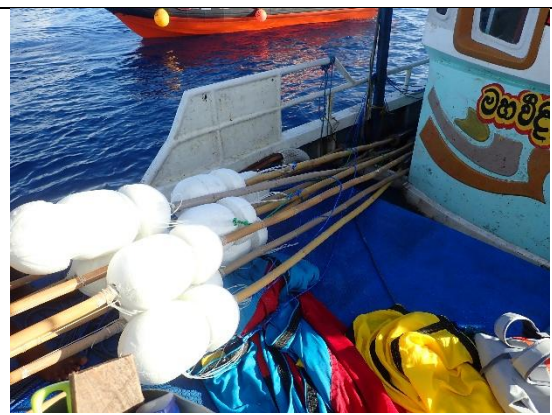
[Fig.10] Fishing gear: danbuoys ready to be set in the water and floating anchor unstowed
