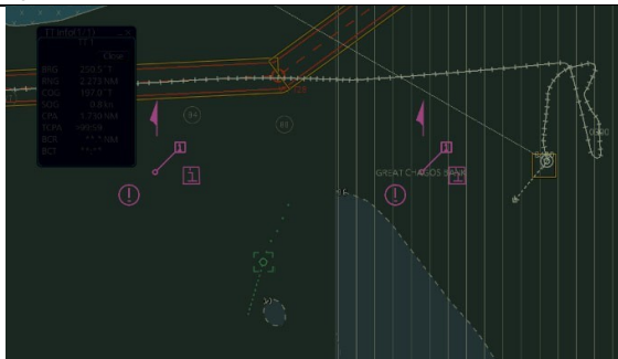
[Fig.21] BPV's ECDIS screenshot taken at 2:17: FV heading North (green marker), speed 4.2knots.
