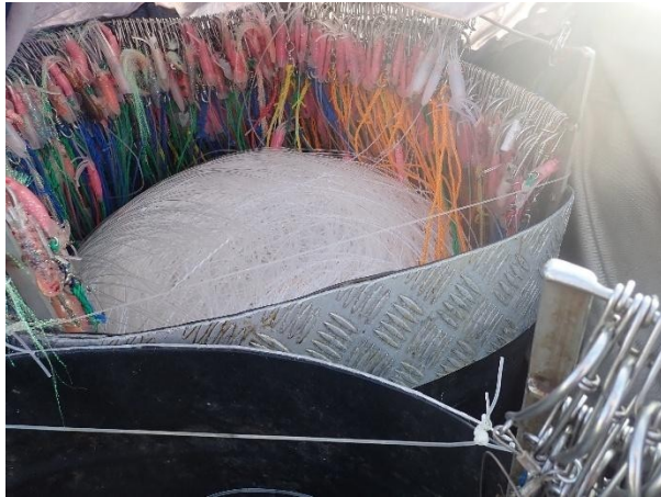
[Fig. 40] Fishing gear, one of two drums with hooks with squid-shape lures.
