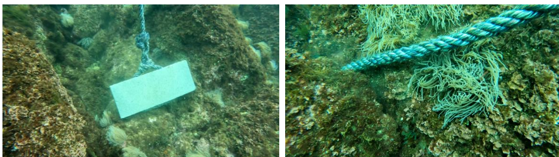
Figure 18. Interaction of the brick ballast and line of the Raft-type dFAD with the seabed.
