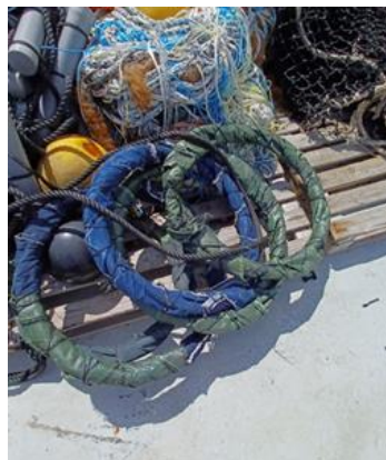
Figure 5 – Typical ballast on a raft-type dFAD, consisting of a metal purse-seine wire ring covered with synthetic canvas.
