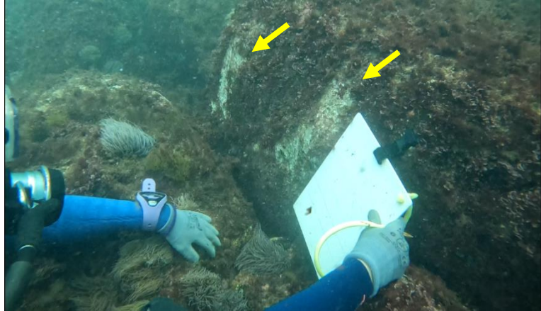
Figure 21. Abrasion damage (indicated with yellow arrows) caused by the lower part of the Cage-type dFAD in contact with the seabed.
