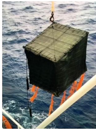
Figure 2 – Cage-type dFAD being deployed in the Indian Ocean (left) and a schematic drawing of a Cage-type dFAD (right).
