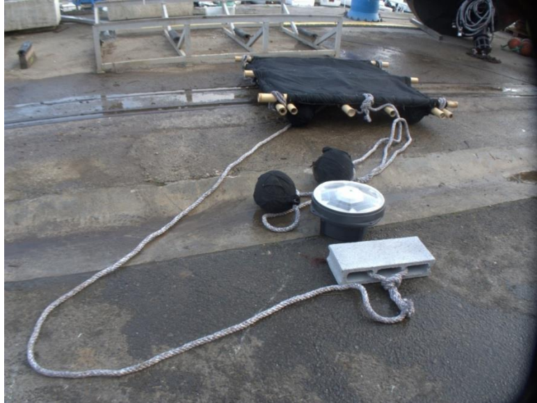
Figure 6 – Raft-type dFAD with a concrete block ballast.
