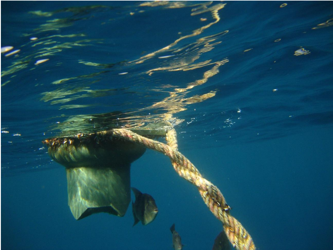
Figure 12. Cotton rope used for the flotation component and geolocating buoy attachment found in perfect condition (photo credit: Joaquín Salvador)
