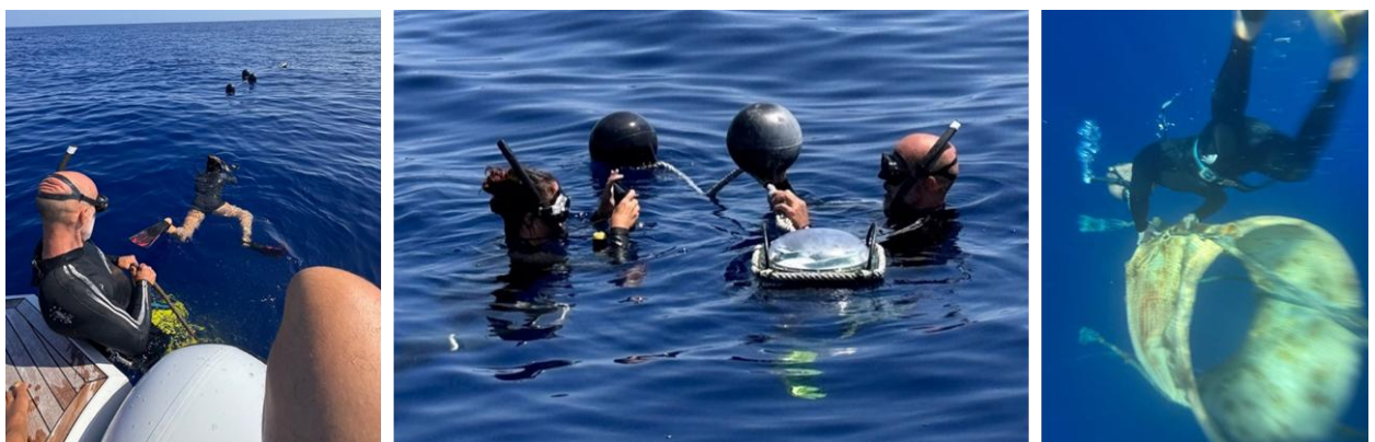
Figure 8. Bio-FAD inspection in the Mediterranean testing. Left - Retrieving the bio-FAD to inspect the main rope. Found in perfect condition both at the surface and at the deepest section of the dFAD; middle – Attachments for the plastic floats found in perfect condition for the two Jelly-FADs
