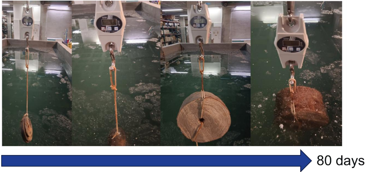
Figure 2. Evaluation of the buoyancy of Paulownia wood in the laboratory. Testing period of 80 days.
