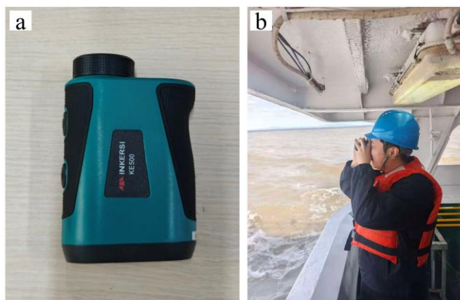
Figure A1 Aerial extent measurement equipment and field measurement procedure for the tori line (a: the INKERSI KE500 visual laser rangefinder; b: researchers measuring the aerial extent in the field)
