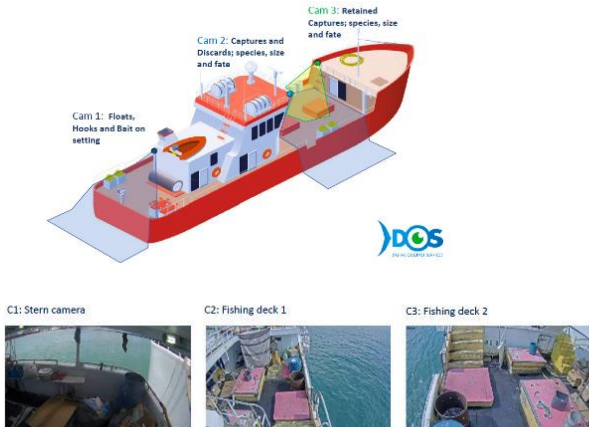
Figure 2. An example of a 3-camera EM equipment installed on a longline covering main areas of fishing and fish handling operations. View of the 3 cameras: (left panel) Stern camera - setting longline providing information on hooks, floats, mitigation techniques and bait; (middle panel) Fishing deck 1 - hauling information, captures and discards, species ID, size and fate; and (right panel) Fishing deck 2 - fate of the species, size, species ID (source: Digital Observer Services).
