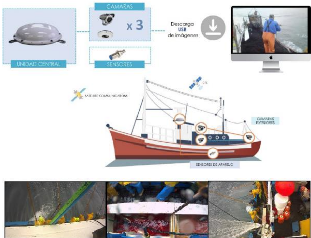
Figure 3. An example of a 3-camera EM equipment installed on a Bay of Biscay (Atlantic Ocean) pole and line vessel covering main areas of fishing activity and fish handling operations. View of the 3 cameras: (left panel) Vessel bridge camera stern view – pole and line activity; (middle panel) Fish handling - catch storage; (right panel) Vessel bridge camera bow view - bait and pole and line fishing activity (source: Marine Instrument.)
