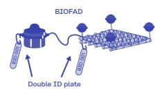
Drawing of the procedure to attach the BIOFAD ID number shown in the metallic plate to the raft and associated echo-sounder buov.
