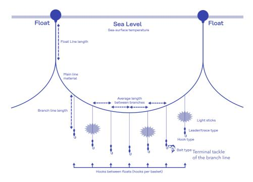
**Figure 1.** Longline (Gear Configuration): Average branch line length (meters): straight length in meters between snap and hook.
