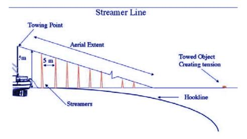
Figure 1. Diagram of Bird Scaring Streamer Line.
