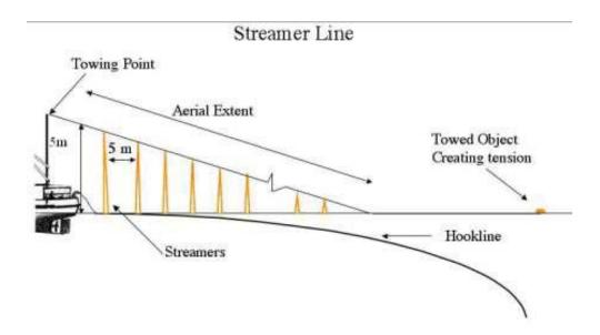
Figure 1. Diagram of Bird Scaring Streamer Line.
