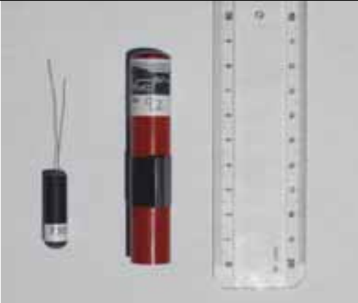
Figure 33: Two types of Vemco sonic tags (FADIO, Dagorn, 2003)
