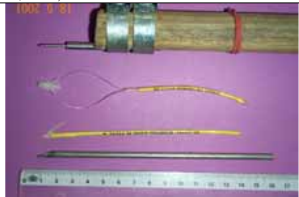
Figure 16: Applicator for Bety tag attached to a wood pole (top) Bety tag (second from top) Dart tag (third from top) Applicator for dart tag (fourth from top) Measuring plastic rule as scale (IRD, MAC, Hallier and Gaertner, 2002)
