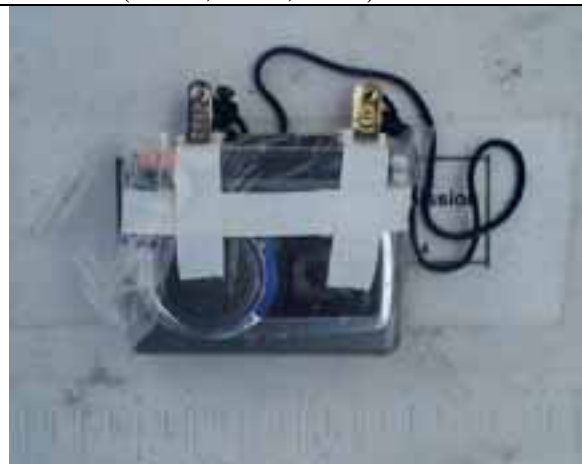
Figure 21: Mini cassette recorder in plastic bag and neck strap ready for data recording. (IOTC, Itano, 2002)
