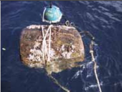
Figure 29: Drifting wood Log or FAD with a radio beacon SERPE buoy (IRD, Tagfad, Hallier et al., 2003)
