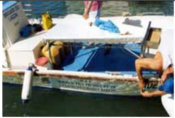
Figure 14: Fitting a large SPC style tagging cradle on a small catamaran (IOTC, Hallier et al., 2002)
