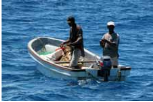
Figure 1: Small open fibreglass boat used for tuna fishing (handline and troll line) in Mayotte (IOTC, Wendling and Million, 2004)
