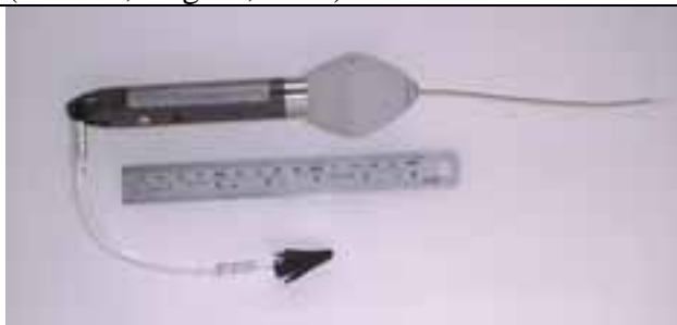
Figure 33: Two types of Vemco sonic tags (FADIO, Dagorn, 2003)
