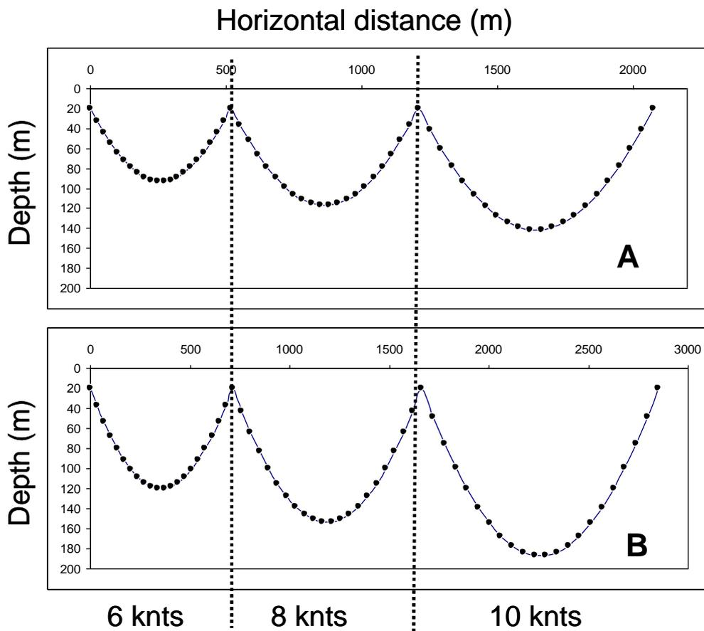
Figure 4 – Variations of the theoretical maximum fishing depth of the mainline for similar baskets in terms of both HBF = 20 hooks and the sagging rate = 0.95 according to different time intervals between hooks (A = 8 s, B = 11 s) and setting speeds of boat (6 knts, 8 knts and 10 knts).
