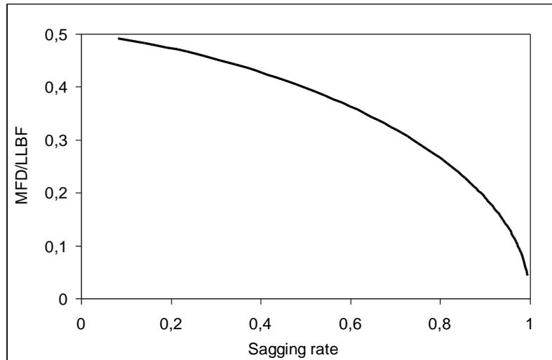
Figure 2 – Theoretical relationship between the ratio MFD/LLBF and SR ( $0 < SR < 1$ ). MFD is the theoretical maximum depth, LLBF is the length of the mainline between floats and SR is the sagging rate. On this figures the value of the length of floatline (LF) and the length of branchline (LB) is supposed equal to zero (from Bach *et al.*, 2005).
