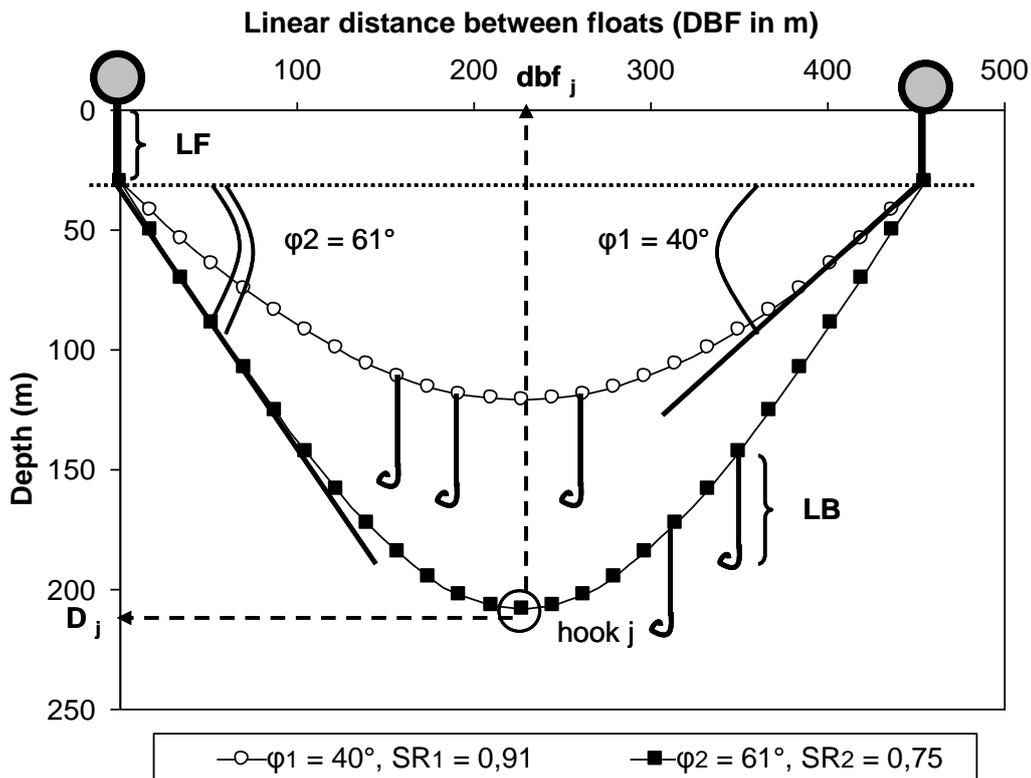
Figure 1 – Theoretical catenary shape of two baskets defined by respective values of the sagging rate of 0,91 ( $\varphi_1 = 40^\circ$ ) and 0,75 ( $\varphi_2 = 61^\circ$ ).  $D_j$  is the depth of the hook j located at a distance  $dbf_j$  from the floatline, LF is the length of the floatline and LB is the length of the branchline (from Bach et al., 2005).
