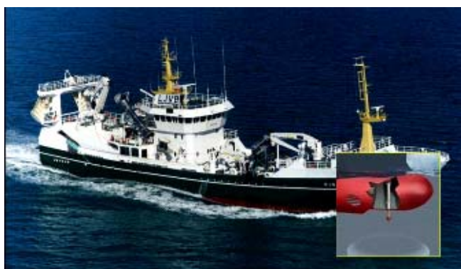
Figure 4a and 4b. Site of omnidirectional sonar on board a fishing vessel: the sonar is generally located in the prow of the vessel (a). Example of fish school detection with the aid of omnidirectional type sonar (b).
