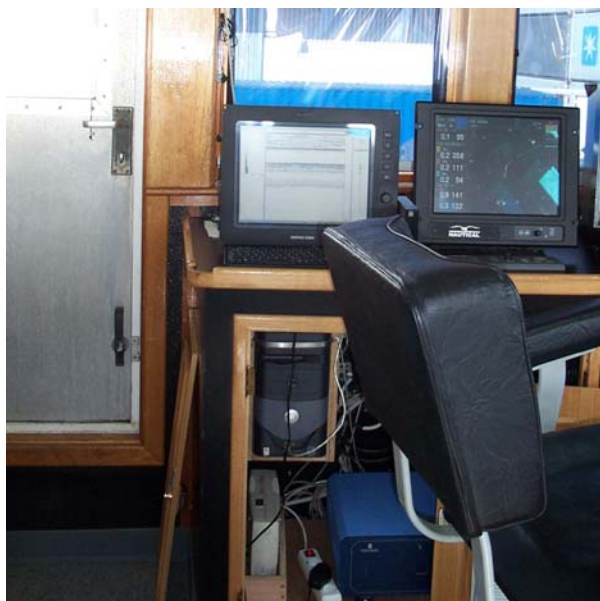
Figure 1. Partial view of the equipment installed on the bridge of the Taraska, and the SIMRAD ES-60 echo sounder with GPS feed.
