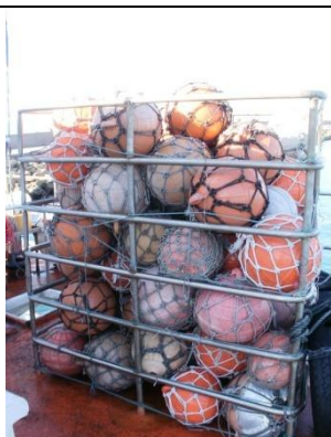
Figure 11. Rigid plastic buoys, mainly used by asian industrial tuna longline vessels.
