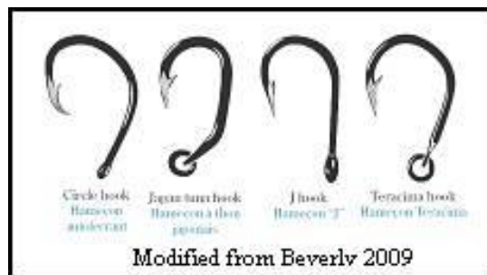
Figure 8. Type of hooks used on longline vessels.
