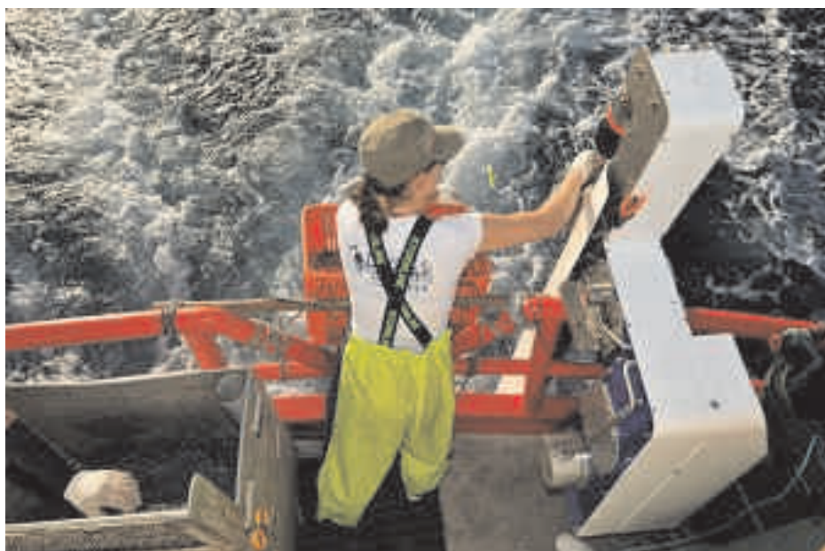
Figure 4. Operating the machine involves two steps – placement of baited hook in capsule and firing the release button on cue from vessel audio beep timer. The release button is the small cylindrical object beneath and slightly to the right of the deckhand's elbow.
