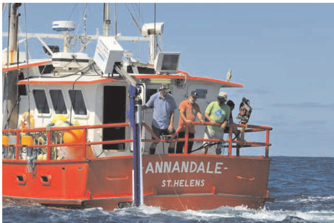
Figure 1. The latest configuration of the Mark 1 underwater setting machine being trialled off eastern Australian in January 2010. The hydraulics and control box are mounted on the roof to reduce the number of pulleys involved in connecting the hydraulics motors to the capsule. Fewer pulleys increase the transfer of energy from hydraulic motors to the capsule, which increases depths attained for a given cycle time.
