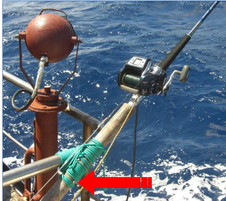
Figure 2. Installation of TDR profiling equipment onboard fishing vessel 'Fournaise'. Arrow shows position of transverse pin for fixation of gimbal butt cap of the fishing rod.
