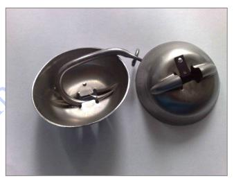
The mild steel shield is hydrodynamic, weighs approximately 38gms and once attached increases the sink rate of the baited hook to 0.6 meters per second, also acting to protect the bait from tearing off the hook when it enters the water after being cast from the vessel.
