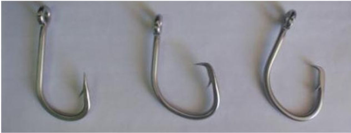
Figure 2: Photograph of the three hook styles used during this study: J hook 10° offset (left); Gt circle hook 10° offset (middle); and G non-offset circle hook (right). Hook measurements in Table 1.
