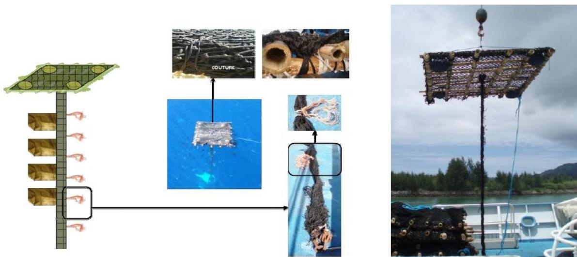
The UHS of this FAD is composed of a single (sometime double) twisted net hanging from under the middle of the raft and weighted by a piece of chain or cable at its bottom end. The net is twisted and braided into a sausage shape, sewn or tied every meter to reduce the likelihood of entanglement. To increase the drift of the submerged structure (which serves as a sea anchor), salt bags and/or small unbraided sections of recycled ropes are attached to the net.
