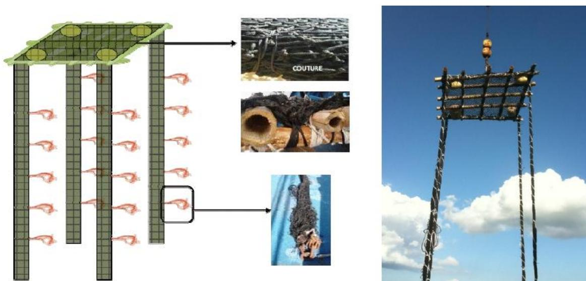
The UHS of this FAD is composed of 2 to 4 strips of net weighted by a piece of chain or cable at their bottom end and attached to each corner of the raft. Each strip is twisted and braided into a sausage shape and sewn or tied every meter to reduce the likelihood of entanglement. To increase the drift of the submerged structure (which serves as a sea anchor), salt bags and/or small unbraided sections of recycled ropes are attached to the ropes.
