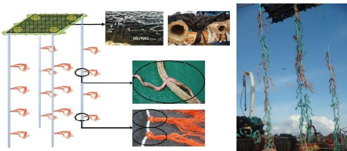
The UHS of this FAD is composed of 1 to 4 recycled ropes weighted by a piece of chain or cable at their bottom end and attached to each corner of the raft. To increase the drift of the submerged structure (which serves as a sea anchor), salt bags and/or small unbraided sections of recycled ropes are attached to the ropes.
